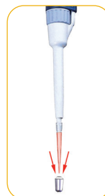
Press FLOWMI onto pipette tip
