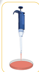
Aspirate sample into 1000µl tip
